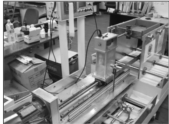
Fig. 6. Durability testing machine.
